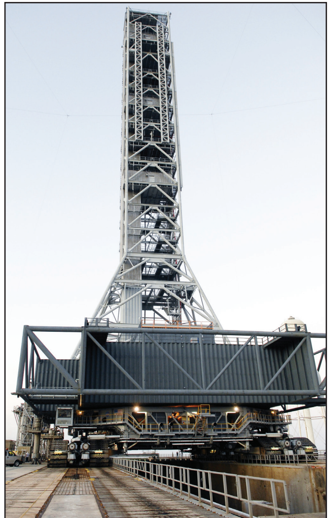
The crawler-transporter, carrying the mobile launcher (ML), completes a 4.2-mile trek Nov. 16, 2011, to Launch Pad 39B at NASA's Kennedy Space Center in Florida.
